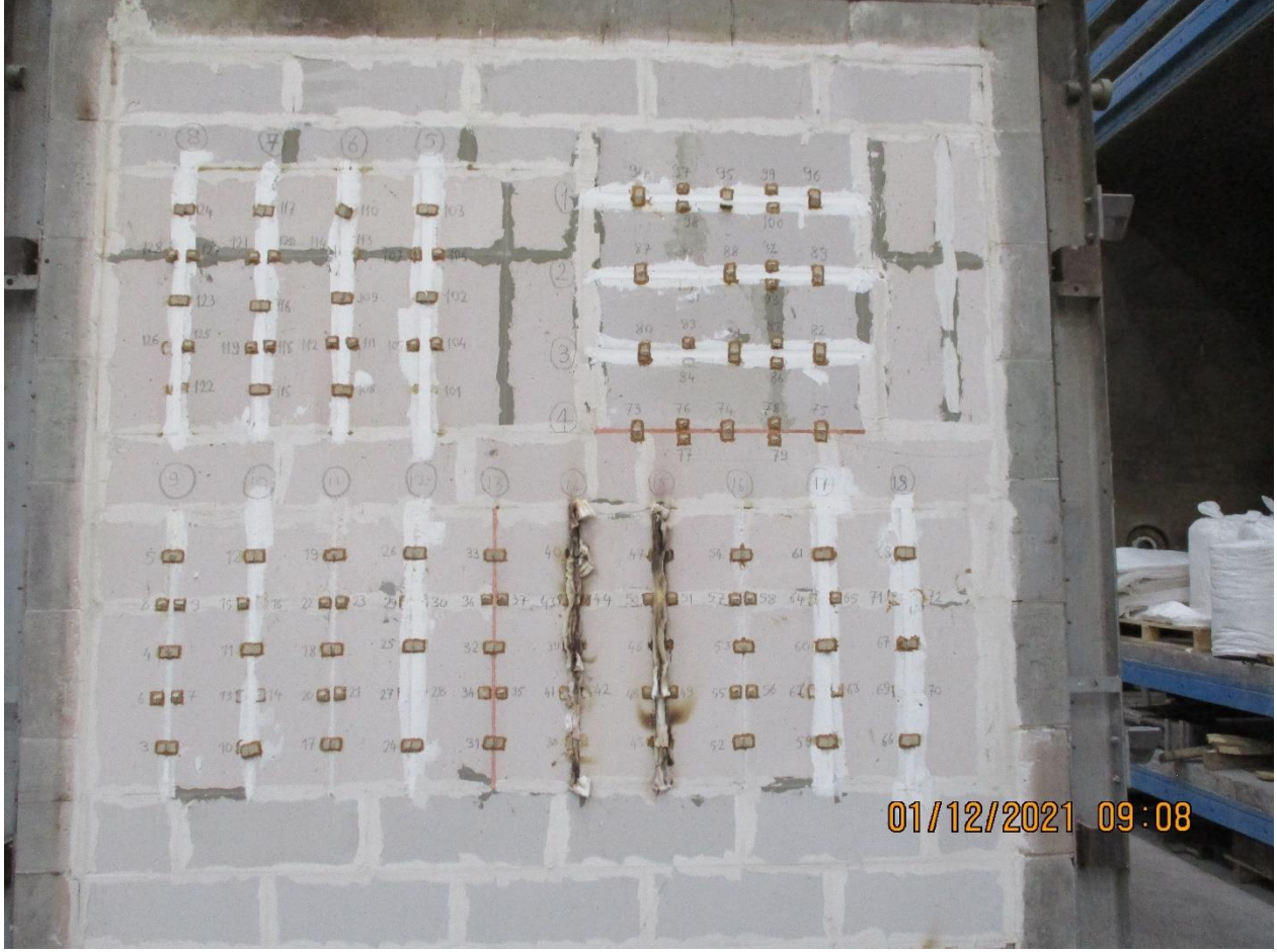
Photo C3: Unexposed side of the test construction after the test.
