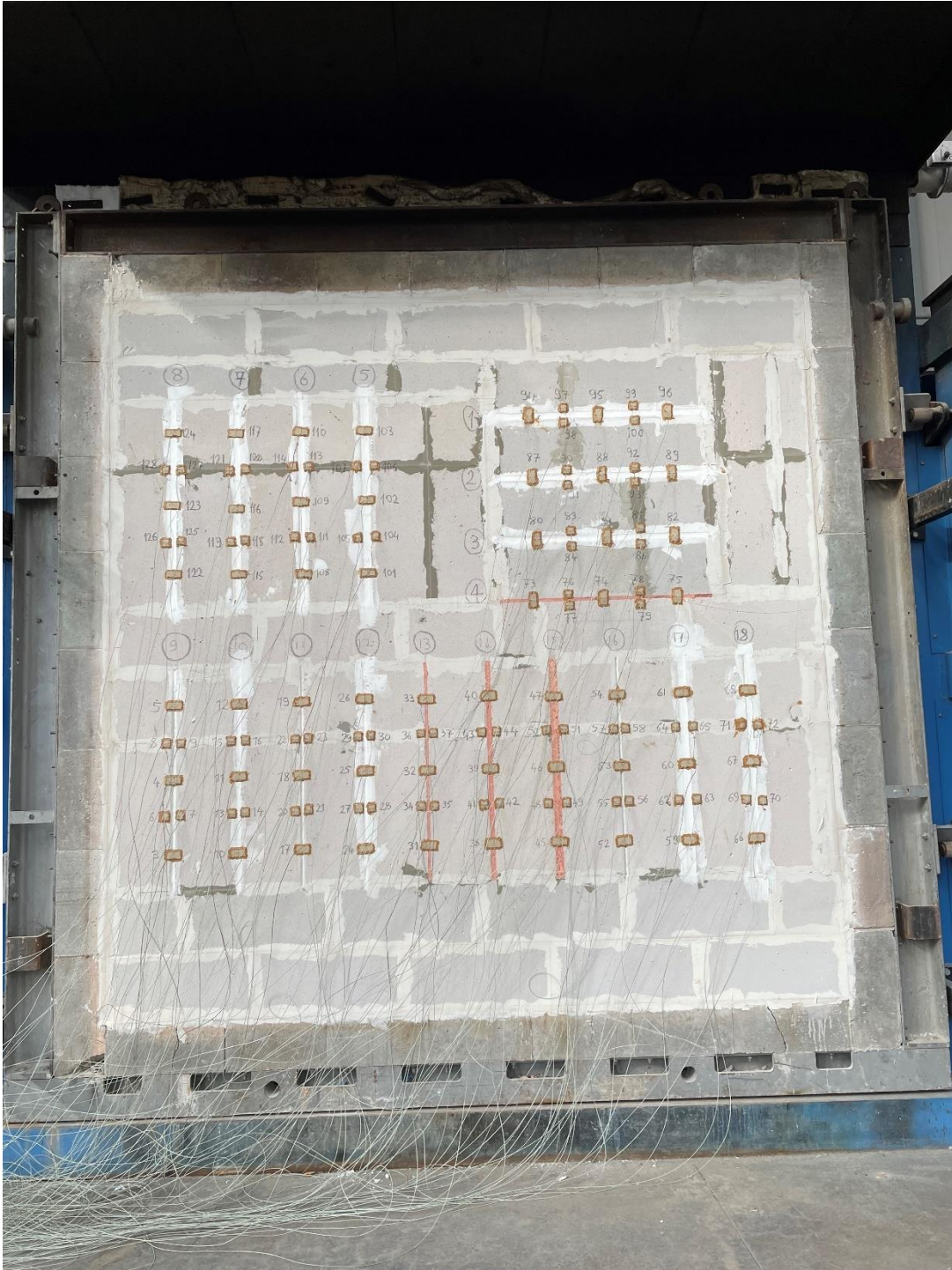
Photo C1: Unexposed side of the test construction before the test.
